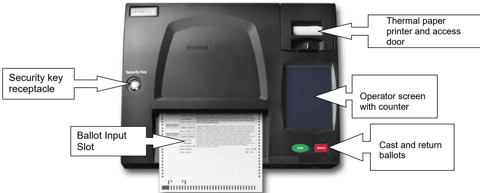
The Above Image shows a Tabulator and its various components including security key receptacle, ballot input, thermal paper printer and access door, Operator screen with counter, and cast and return buttons.
